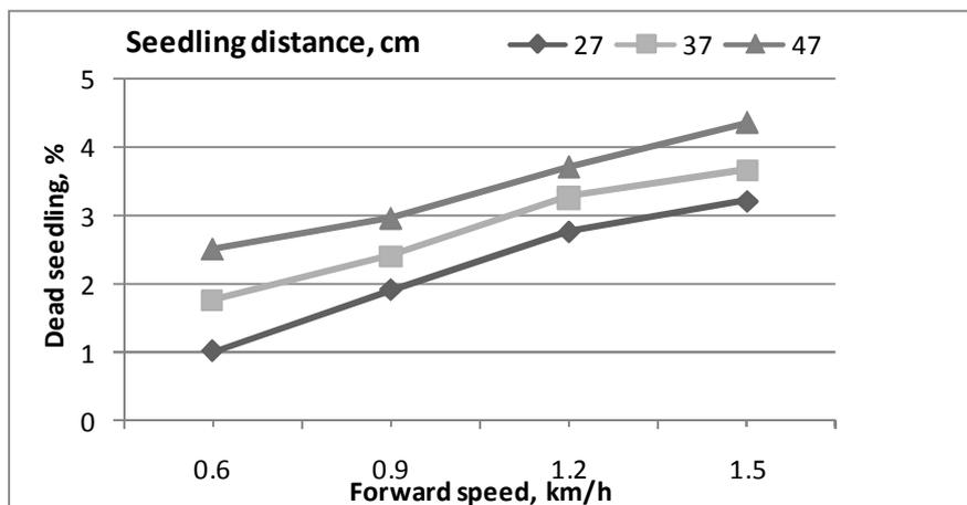
Fig.9. Effect of forward speeds and seedling spaces on dead seedling
