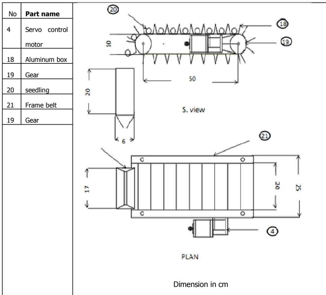
Fig.2. Side and plan views of conveyor belt of transplanting unit.
