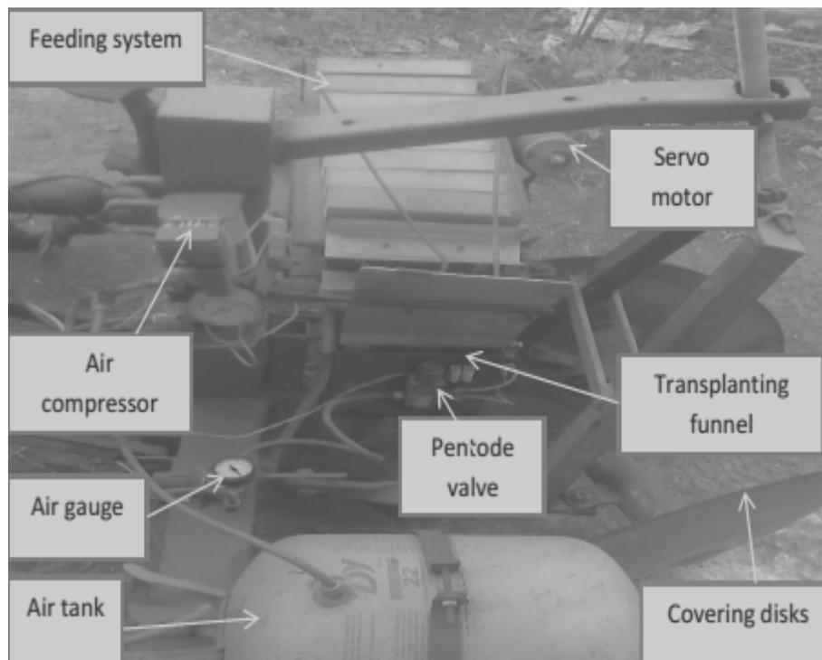
Fig. 3. The main components of the developed transplanting unit.
