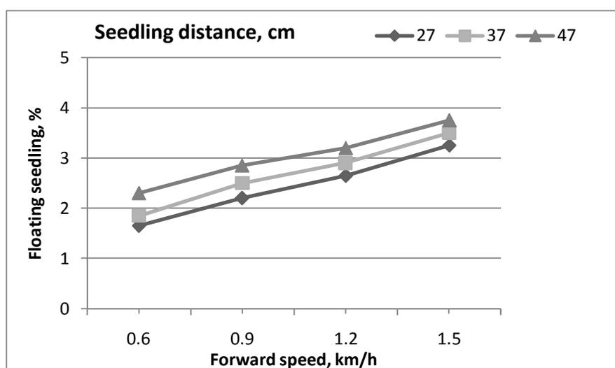
Fig. 8. Effect of forward speed and seedling spaces on floating seedlings.
