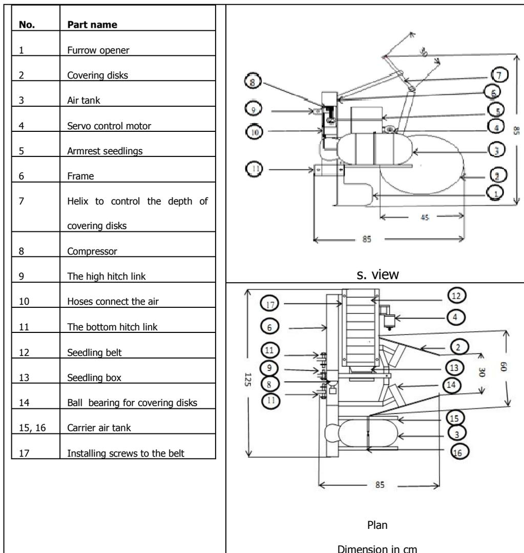
Fig.1. The schematic plan and side views of the transplanting unit.
