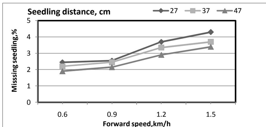
Fig. 7. Effect of forward speed and seedling distances on missing seedling.
