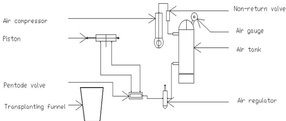
Fig.4. Main components of air circulation.
