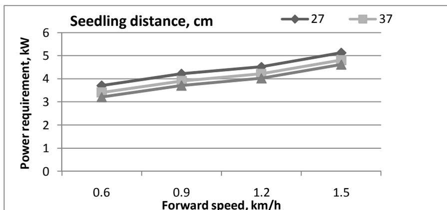
Fig.10. Effect of forward speeds and seedling spaces on power requirement.
