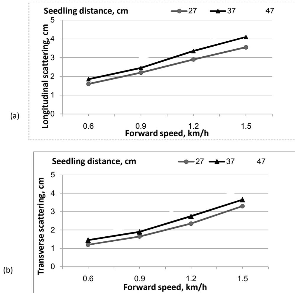
Fig. 6. Effect of forward speeds and seedling spaces on (a) longitudinal and (b) transverse scattering.
