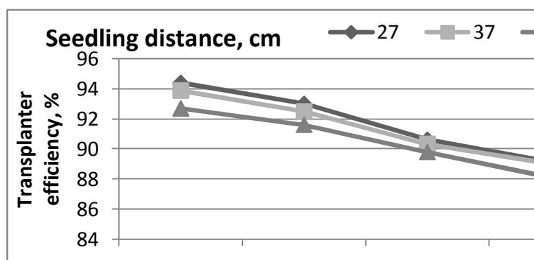
Fig.11. Effect of forward speeds and seedlings spaces on transplanting efficiency.
