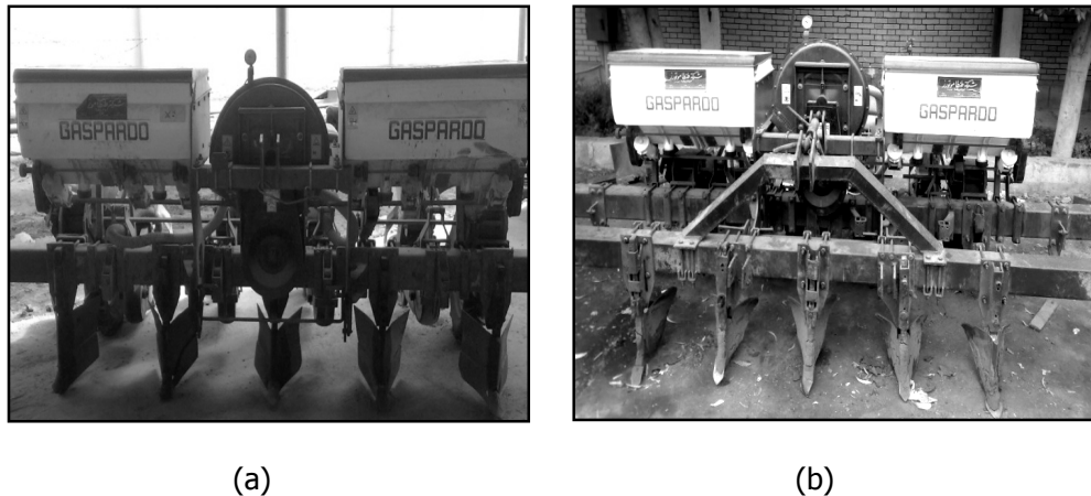
Fig . 2. Photo of the planter before modification (a) and after modification (b).
