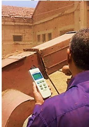
**Fig.4: Measuring airstream velocity by the anemometer.**
