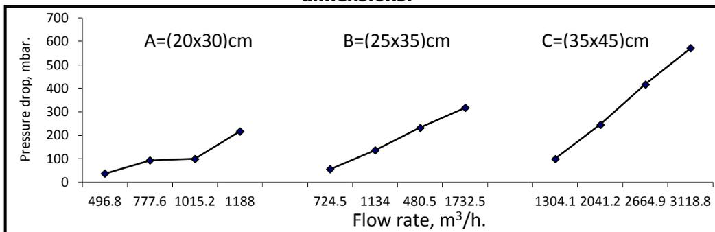
**Fig. 9. The pressure drop versus flow rate at different cyclone inlet dimensions.**
