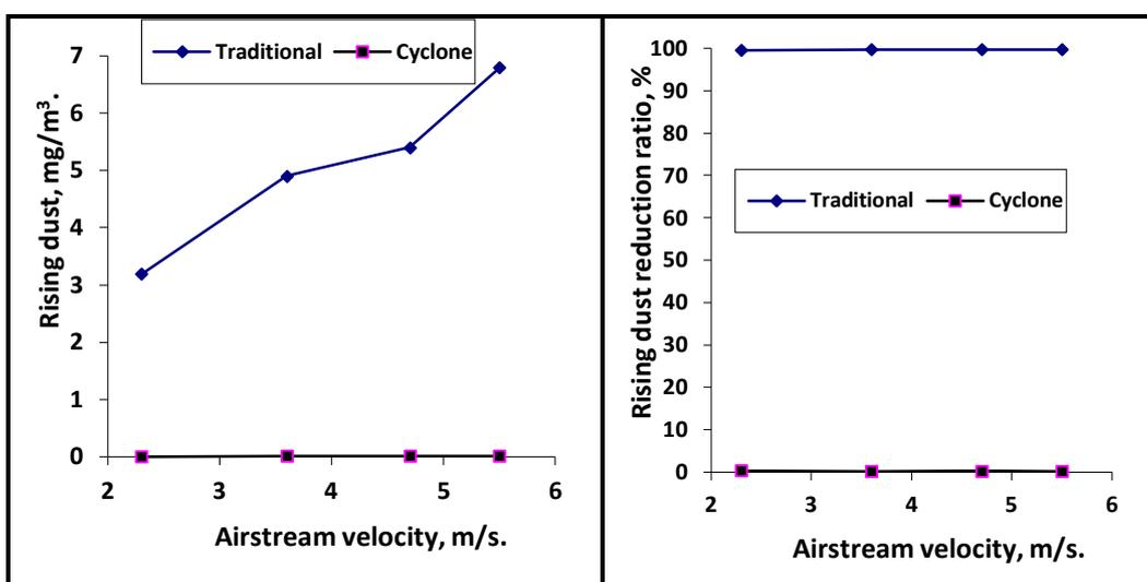
**Fig 10. Effect of airstream velocity on rising dust, mg/m<sup>3</sup>.**
