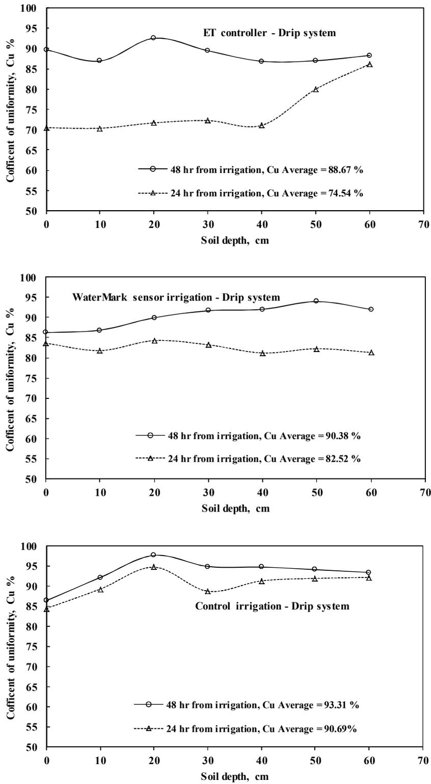
Fig. 2. Values of  $C_u$ s as a function of soil depth after 24 and 48 hours of irrigation, for the three irrigation-scheduling methods
