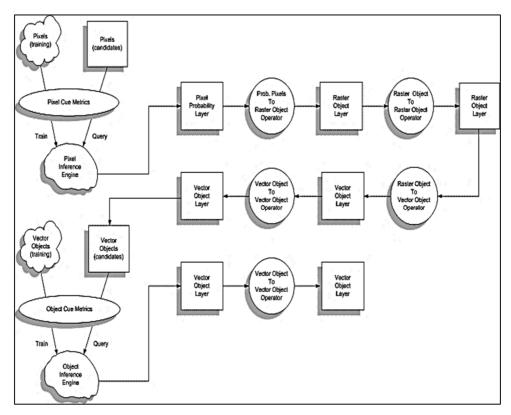
Figure 3. IMAGINE Objective Process Flow Diagram
