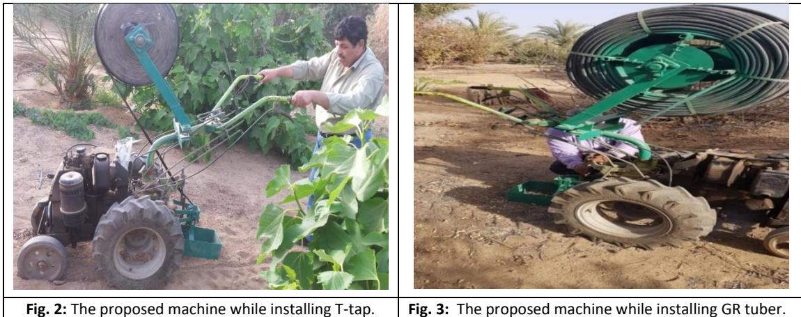
Fig. 2: The proposed machine while installing T-tape.
