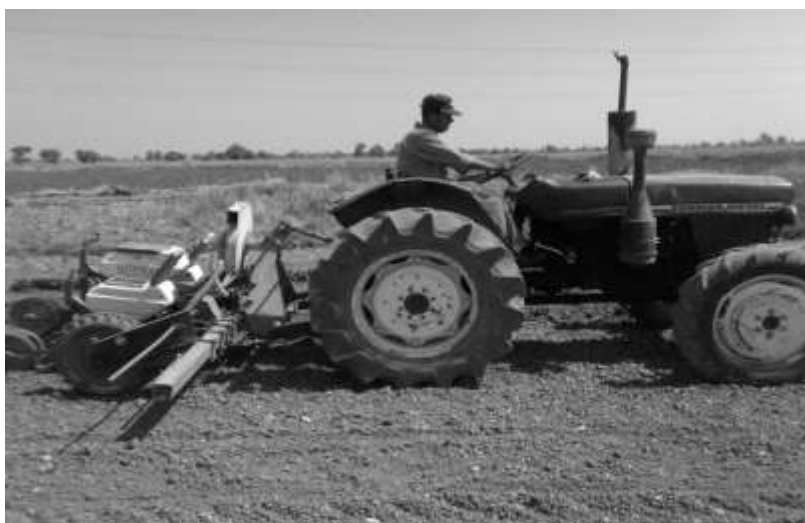
Fig. 4. Yanmar tractor and Koymac precision vacuum planter.
