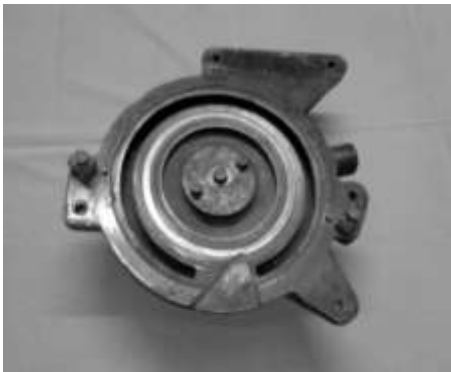
The main shield with air cut-off device
