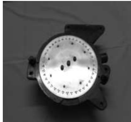
The seed plate inside the shield
