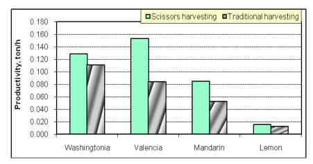
Fig. 9. Effect of using electrical harvesting scissors on the labor productivity of citrus fruits.
