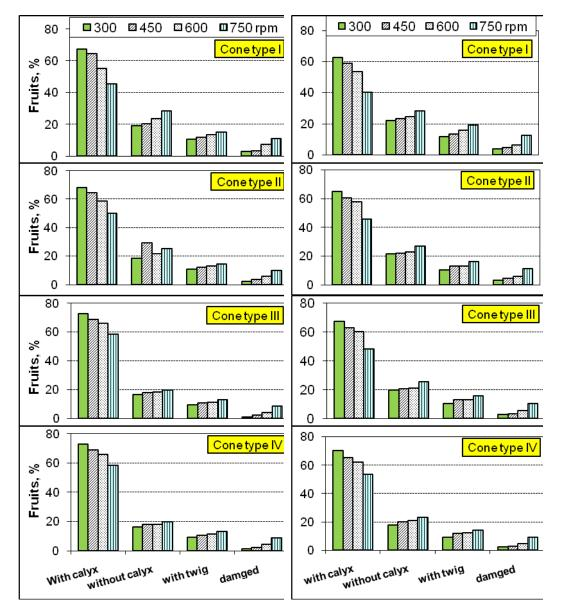
Fig. 8. Effect of using cone harvesting head on the harvesting quality of Washingtonia (left) and Valencia (right) orange fruits.
