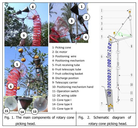
4- Fruit receiving and collecting mechanism: it consists of: a) Fruit receiving telescopic tube which fixed on the housing mechanism to receive the detached fruit and transported it to the collecting basket. b) Fruit collecting basket which attached at the lower end of the receiving tube to collect a citrus fruits detached from citrus tree. This basket is equipped with two wheels to make it easy during moving between trees in field and also, easy to empty.
