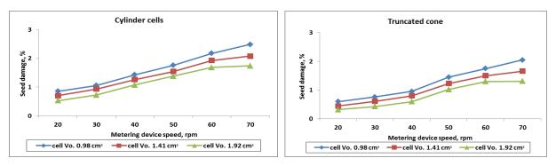
Fig.6. Effect of metering device speed, cells volume and cells shape on seed damages
