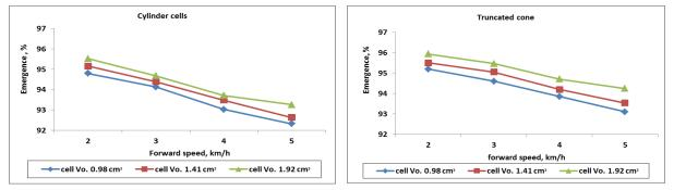
Fig.9. Effect of forward speed, cells volume and cells shape on emergence percent
