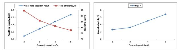
Fig.13. Effect of forward speed on actual field capacity, field efficiency and slip percent
