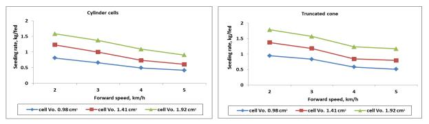
Fig.8. Effect of forward speed, cells volume and cells shape seed discharge
