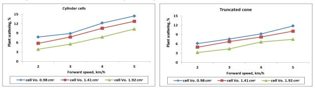
Fig.10. Effect of forward speed, cells volume and cells shape on plant scattering
