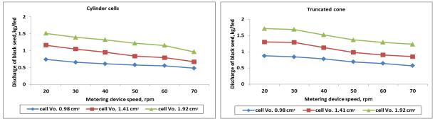
Fig.5. Effect of metering device speed, cells volume and cells shape on seed discharge
