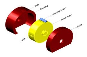
Fig.2. colored isometric of the metering device
