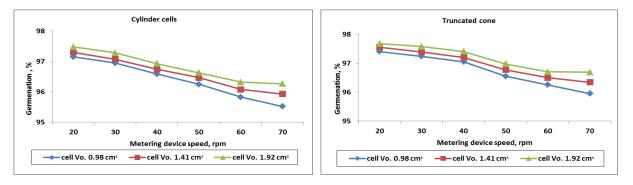
Fig.7. Effect of metering device speed, cells volume and cells shape on germination percent
