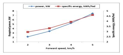
Fig.14. Effect of forward speed on required power and specific energy
