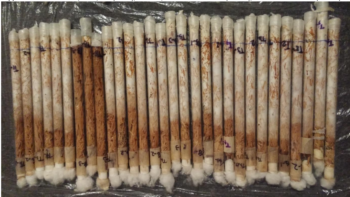
Fig. 1. Mycelia growth in 15-cm glass tubes. Showing a photograph of the glass tubes. The length of the white covered area of mycelium in each tube was measured considering the marked line as the origin of coordinates.
